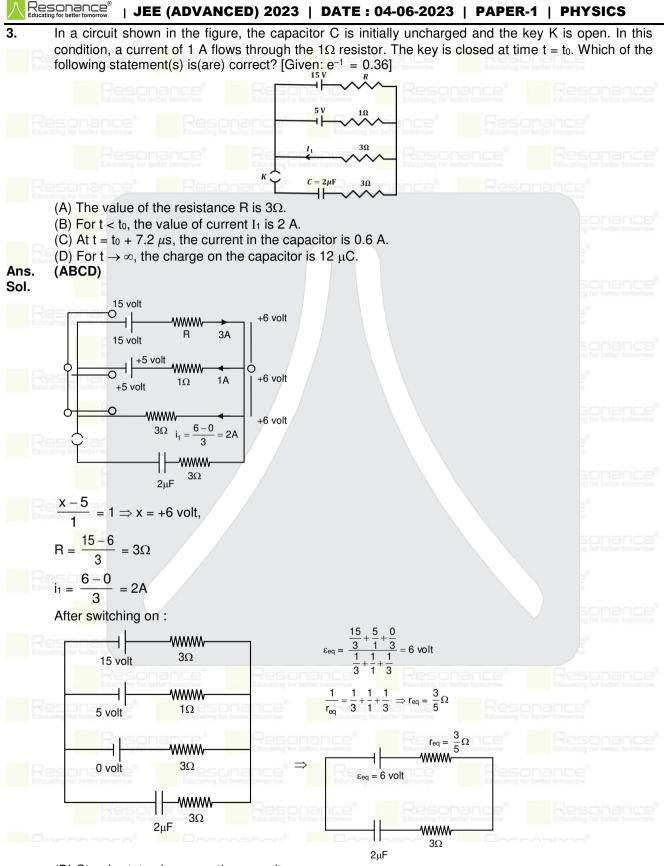
(D) Steady state charge on the capacitor
